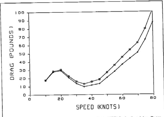
Figure 7 This figure shows the upper and lower bounds on drag produced by the "DELTA-Drag" scaling technique. The true drag of the craft lies somewhere between the two lines.
