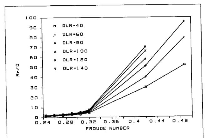
Figure 2 This figure reproduces Skene's version of the Taylor series data. DLR is the displacement/length ratio. The drag is expressed as pounds of residuary drag per ton displacement.
