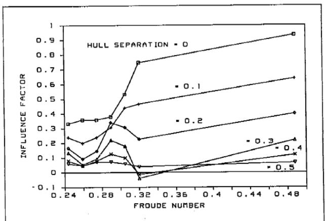
Figure 1 This figure reproduces the data presented by Turner & Taplin in 1968. "Influence Factor" is the drag augment due to hull spacing. "Hull Separation" is the clear distance between hulls expressed as a fraction of length.
