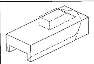
Figure 12 This figure shows the definition of "SES Cubic Number." This pseudo-volume is the volume of a rectangular prism that circumscribes the hull, minus the volume of a prism circumscribing the cushion.
