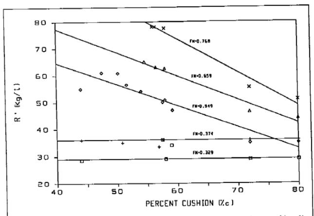
Figure 5 The Simplified Method (Eq'n 3a-e) for SES drag assumes that resistance can be related to the percent of the craft's weight that is carried by the cushion. The lines are fit through experimental data. The equations are in the text.
