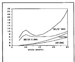
Figure 4 This plot graphically depicts the drag breakdown used in the drag prediction method called "reliable." The key to this technique is the definition and scaling of the component called "Delta" drag.
