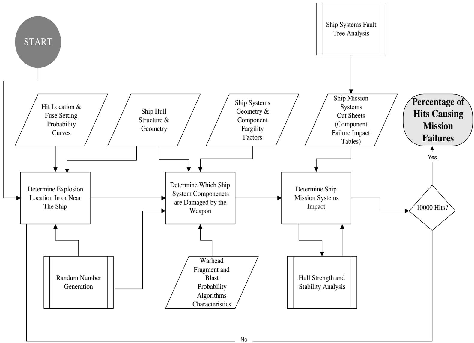
Figure 1 - JJMA Ship Vulnerability Simulation Model
