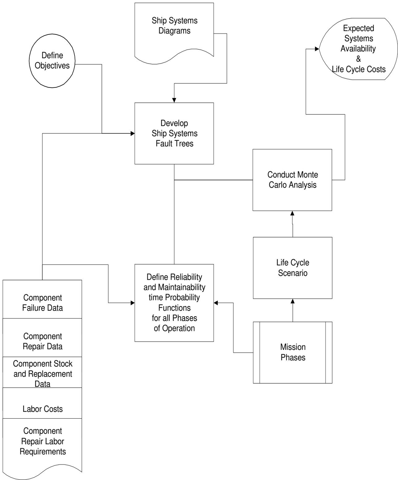
**Figure 2 - The Process for Development of the Ship Systems Availability and Life Cycle Cost Analytic Model**
