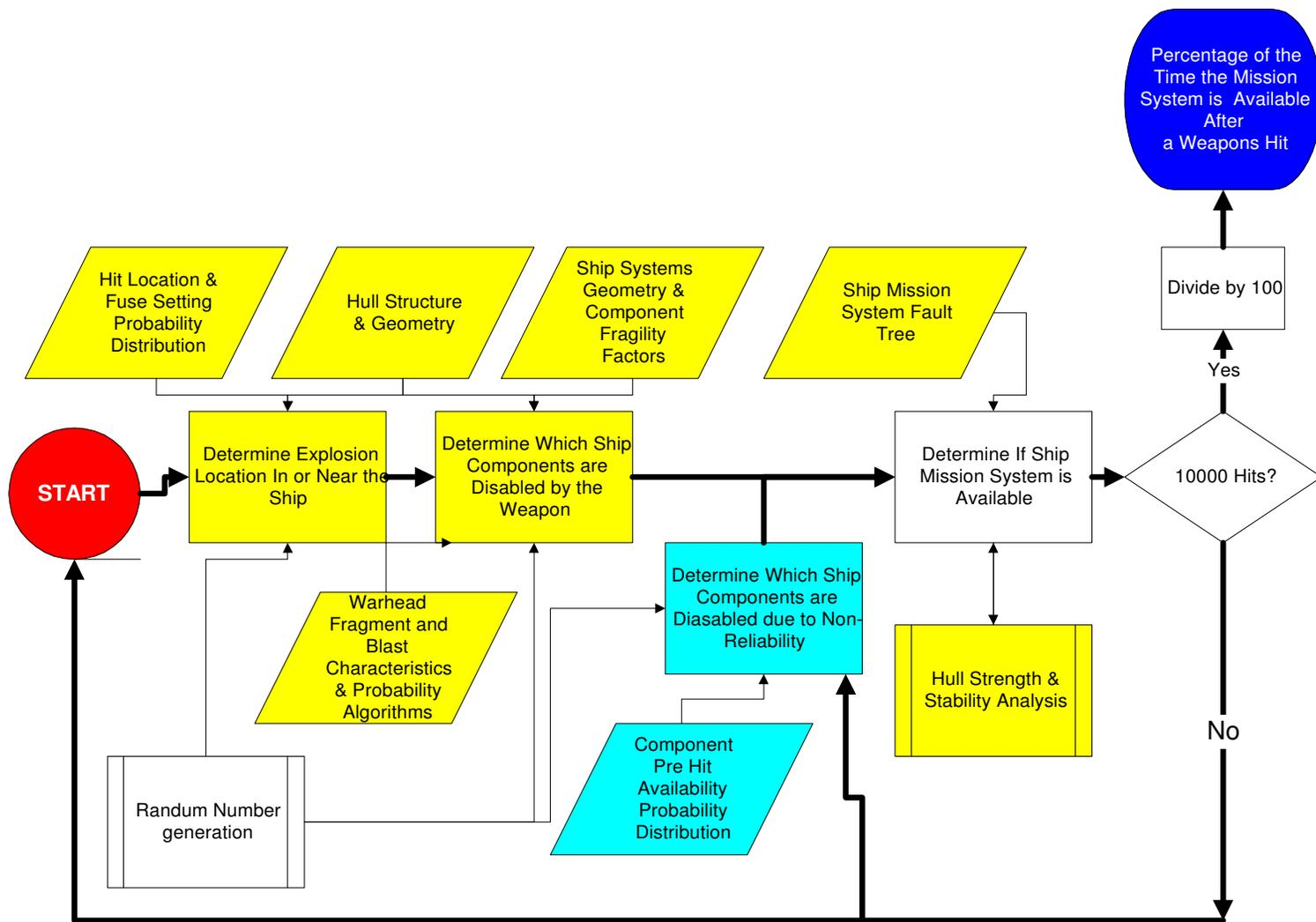
**Figure 1. Process for Assessing the Effects of Component's Deactivation on Systems' Availability after the Hit.**
