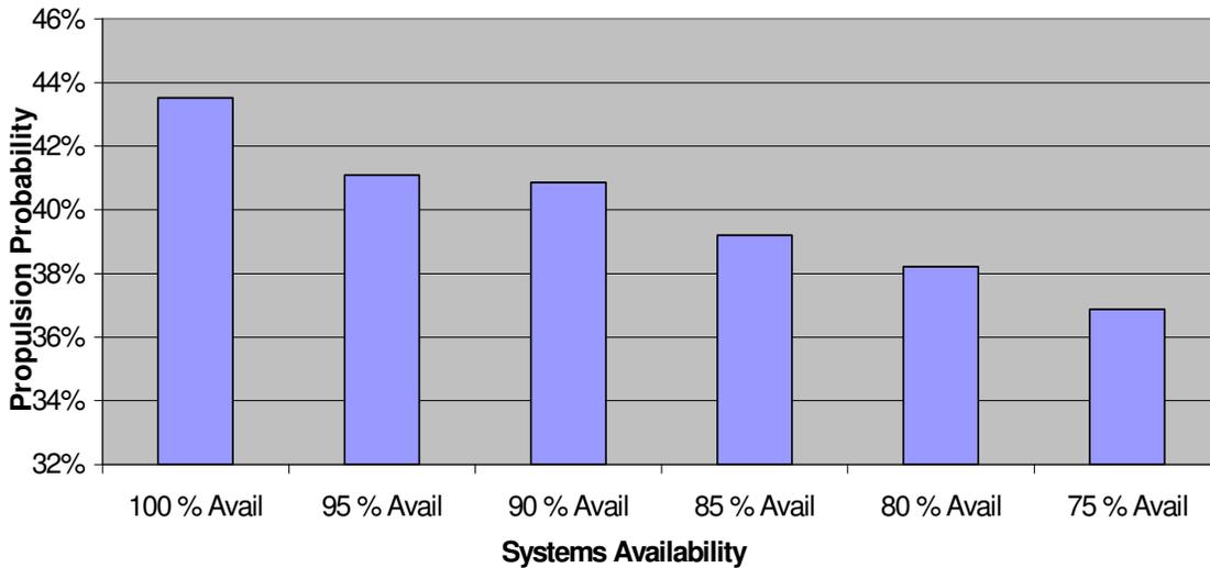
**Figure 9 - Probability of Having at Least 50% of Ship’s Propulsion Available
