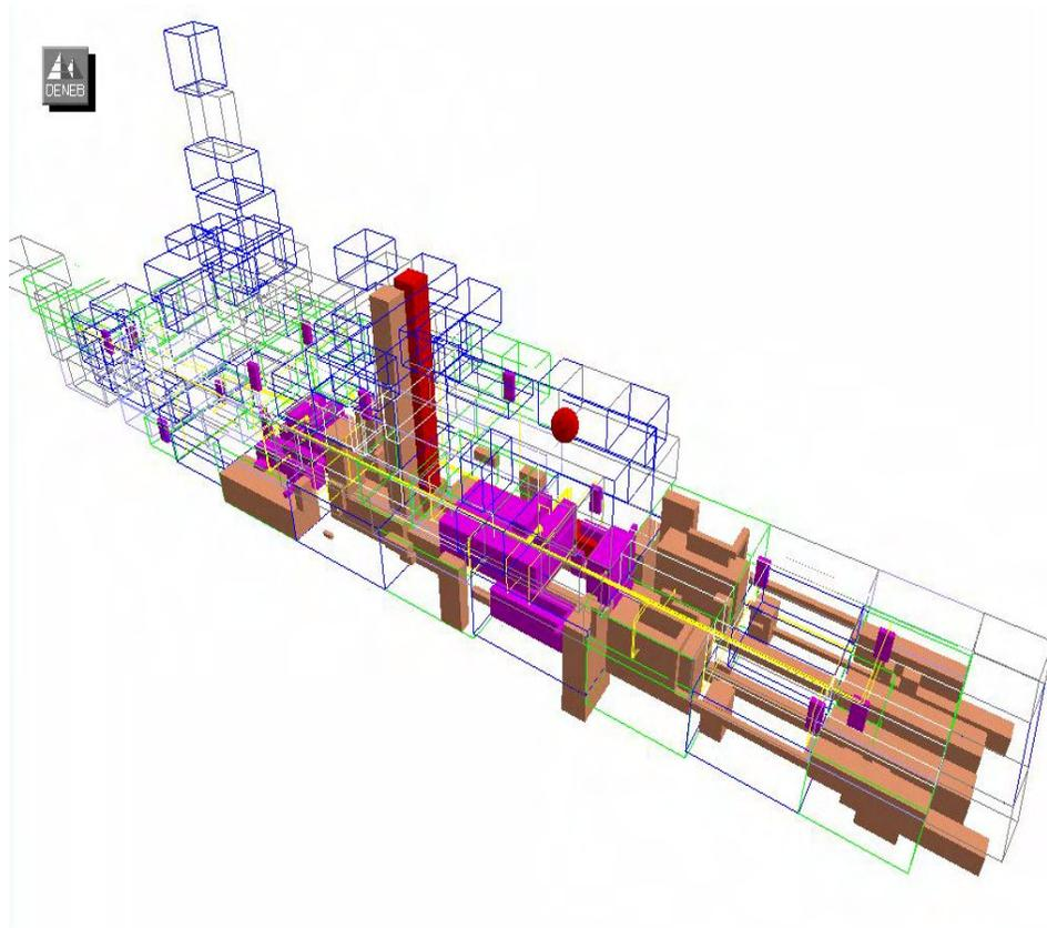
**Figure 4 - JJMA SVM Graphic of a Small Combatant Propulsion Plant under SAP Attack**
