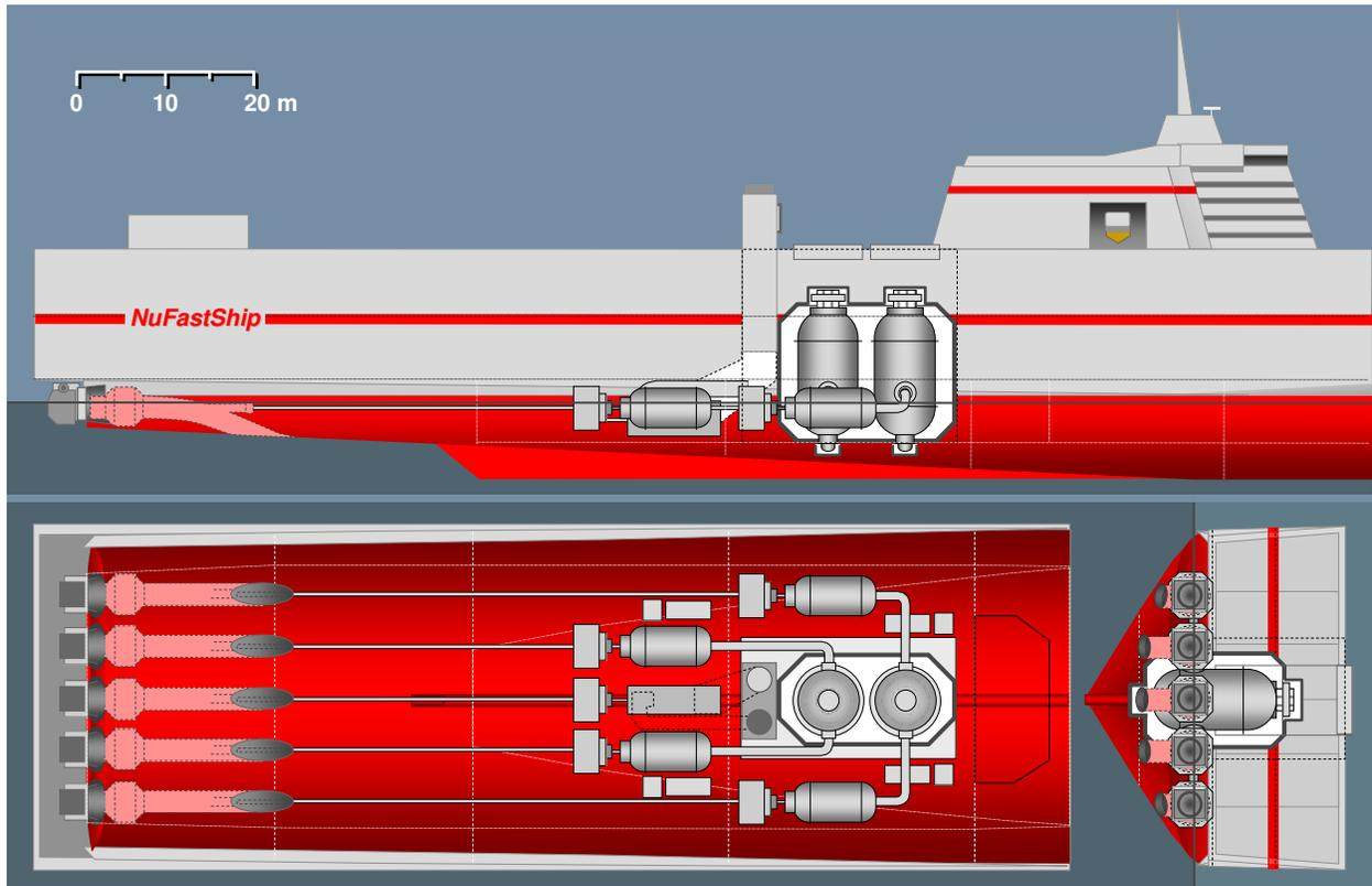
Figure 7 Nuclear-Gas Turbine Propulsion Plant Layout for “FastShip”
