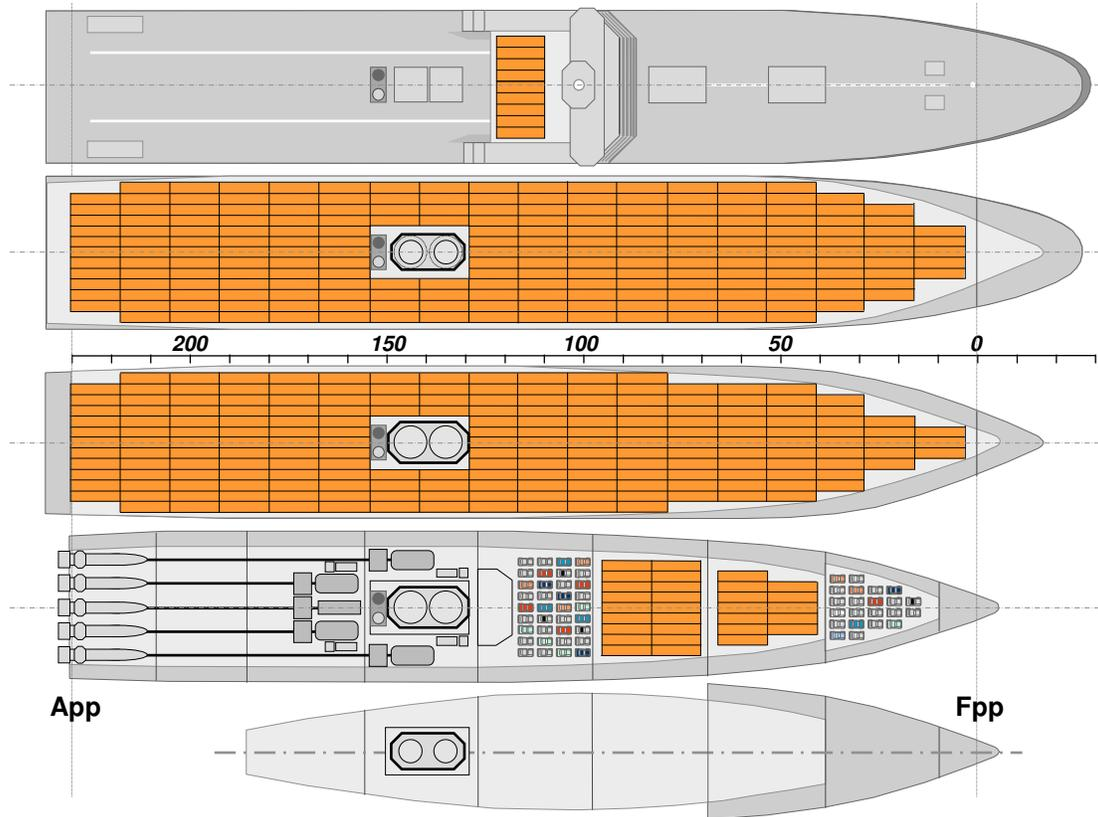
**Figure 8 Cargo Arrangement for the Hybrid “FastShip”**
