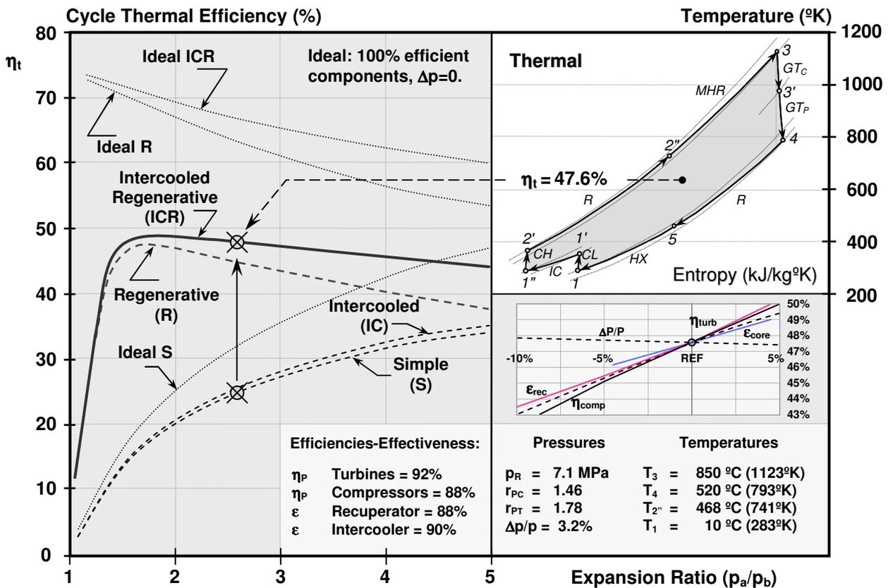
Figure 2 Thermal Efficiencies of Brayton Helium-Closed Cycle Options
