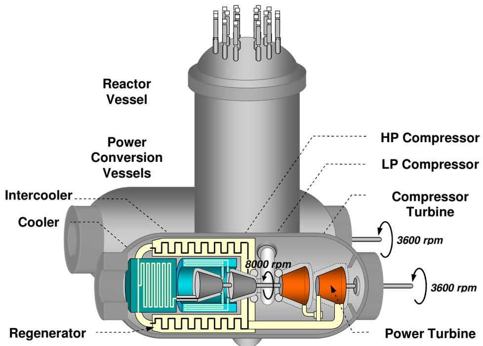
Figure 5 represents the internal arrangement of a PCV, in which the gas expands through the compressor turbine spinning at about 8,000 rpm, and through a power turbine. Power level control is provided by gas pressure adjustment at nominal efficiency, and by a power turbine by-pass.
