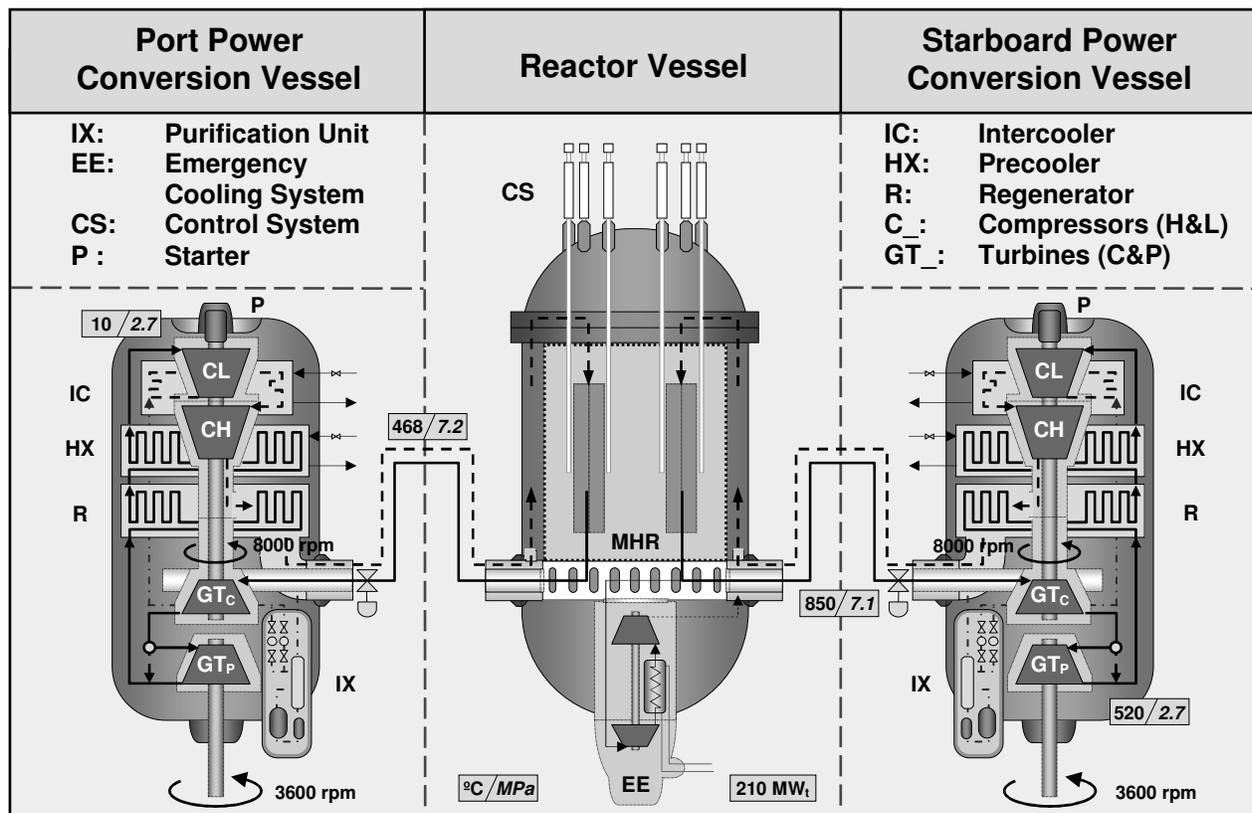
Figure 6 Helium Flow Circuit in a GT-MHR Propulsion Plant Module
