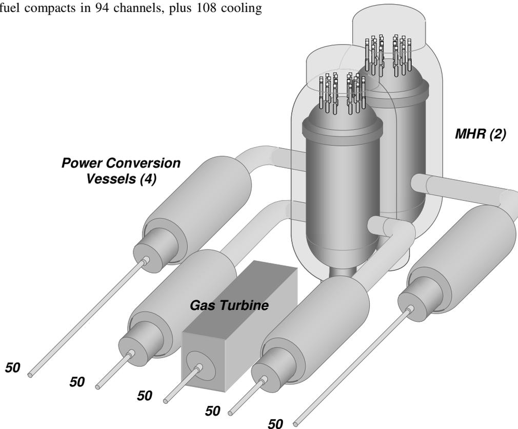
Figure 3 Hybrid Propulsion Plant (Nuclear-Gas Turbine)
